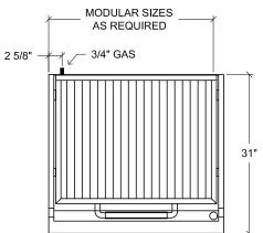
27" clearance required in front for removal of grease container
