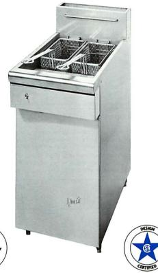
The MV40 features S.S. radiants and rugged powerful but quieter burners. The all welded stainless steel tank has 40 lb. (18 kg) fat capacity and is the "easiest to clean" tank made. The deep cool zone with crumb catcher keeps burned particles away from cooking heat to prolong fat life. The stainless steel fryer front and unique open base combine to make drainage simple and permit thorough, easy cleaning.
